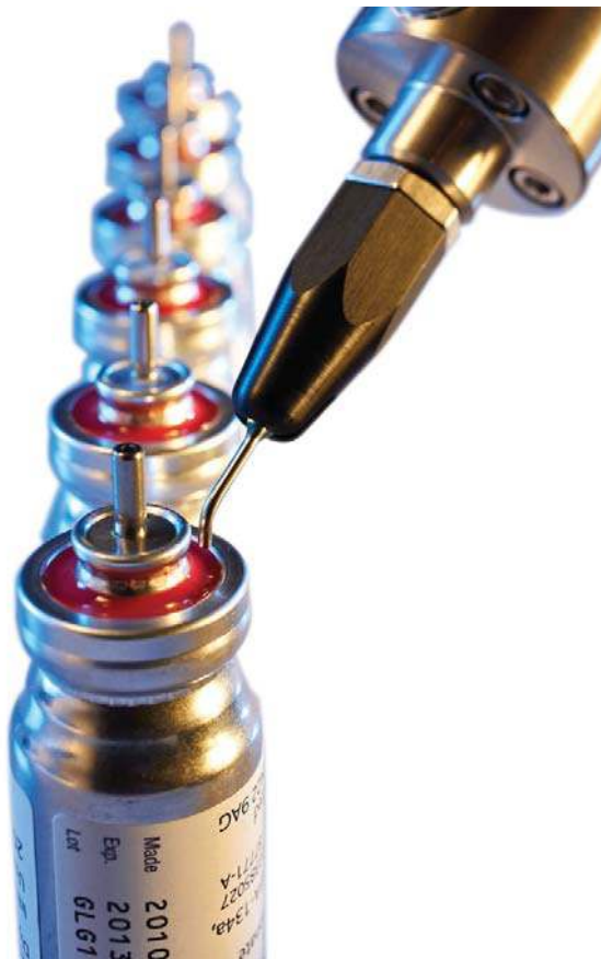
TS55440 - Dispensing medical device adhesive
