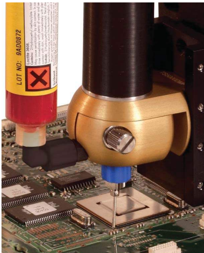
TS5000DMP - Performing underfill
